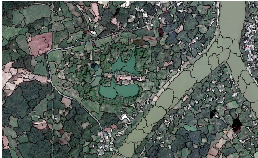
Fig. 3. A sample of image segmentation at Scale of 10, Shape of 0.75, and Compactness of 0.5 for a SPOT satellite image acquired in 2016 at the Minh Mạng Tomb (H11).
